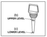
If oil level is below the lower level line (c), refill with suitable oil (see table) to upper level line (b). Do
