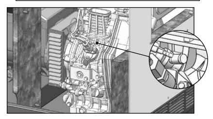
If the fuel filter or the fuel hoses get air, it is necessary to disconnect the Diesel hose close to the injection pump and drain it.
