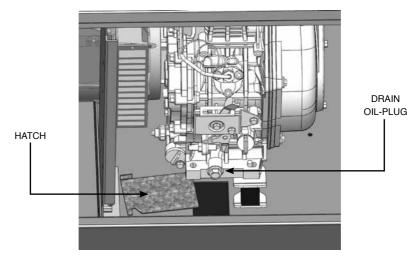
Use new and high quality lubricating oil to the specified level as mentioned in the page 10. If contaminated oil or deteriorated oil is used or the quantity of the engine oil is not sufficient, the engine damage will result and its life will be greatly shortened.
